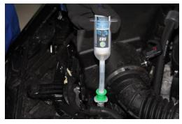
7. Afterwards disconnect quickly the adapter system from the AC service point.
