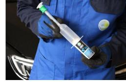
5. Wait at least for 1 minute with the engine running (see step 1) before connecting the filling system. Make sure to connection is tight.
