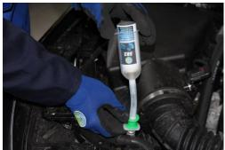
6. Get the engine up to 2000 to 2500 RPM, then press the can TUNAP 582 into the filling adapter until the whole product has been added to the cooling system (around. 5 seconds).
